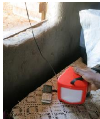
Figure 23 Charging a mobile phone using the S250 solar lantern.
